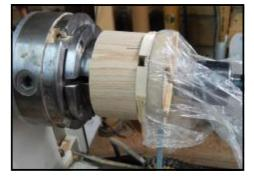
Repeat the process with 6 60 degree segments on the other side of the wheel. Make sure the gaps in the 1st ring of segments are centred on the edges of alternate segments in the 2nd ring as shown here. For the 3rd layer repeat the process with the remaining 3 120 degree segments on the "3" side of the wheel. Again, make sure the gaps in the 3rd ring are centred on the edges of alternate segments in the 2nd ring.
