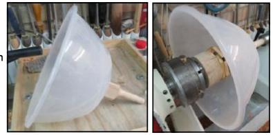
From this point on, the making of the apple is nothing remarkable. For safety, having mounted the larger section of the blank in the chuck, I normally provide tailstock support with a live centre, just until I am confident that the blank is in balance, and it is all holding together.
