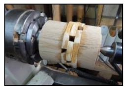
Finally, the second part of the original blank is applied with a live centre holding it in place. Ensure the witness marks are aligned, and apply the glue.
